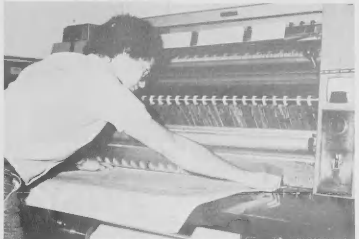
Contractor's employee, W. Yarzagaray, producing copies of a map by using the "bruning" white printer machine.
